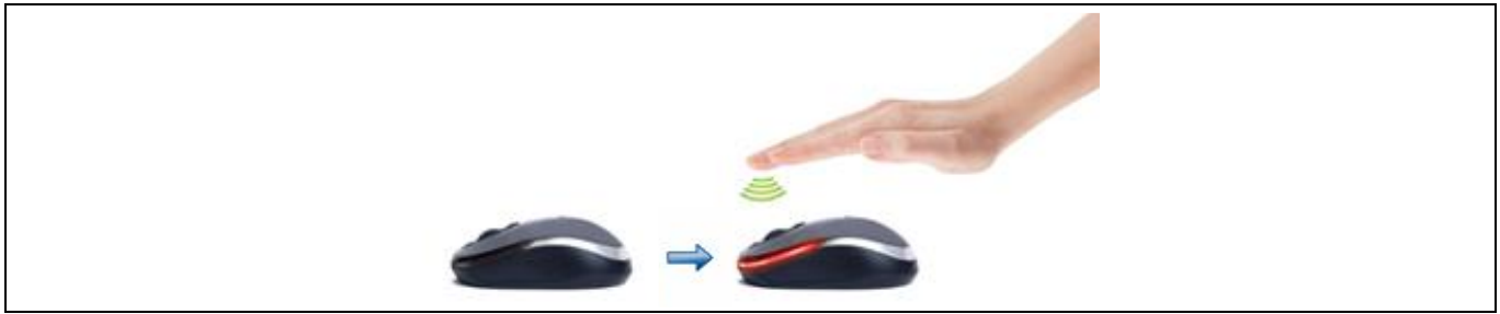
Figure 44 Wake-on-approach implemented in a mouse
