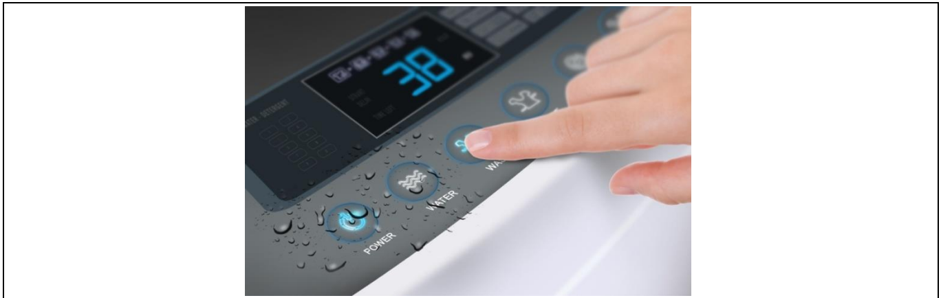
Figure 32 CAPSENSE™-based touch user interface in a washing machine with liquid tolerance
