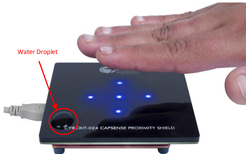
Figure 27. Proximity Detection in Presence of Water Droplet
