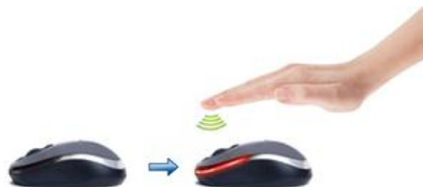
Figure 5. Wake-on-Approach Implemented in a Mouse
